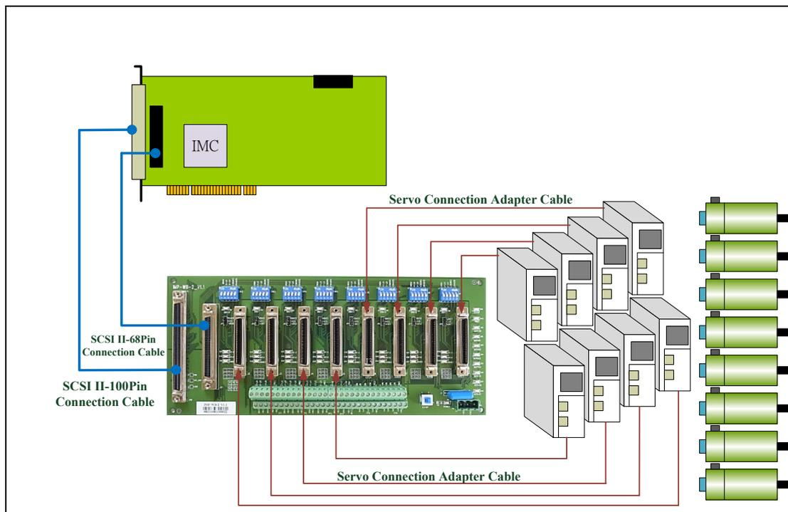
Fig.1-1 System Connection Diagram
